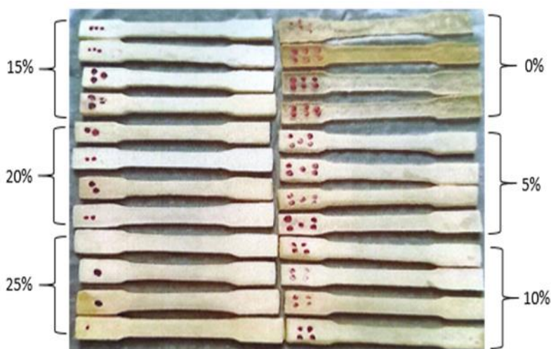
Figure (2): Epoxy samples added with magnesium oxide powder in different weight ratios.
